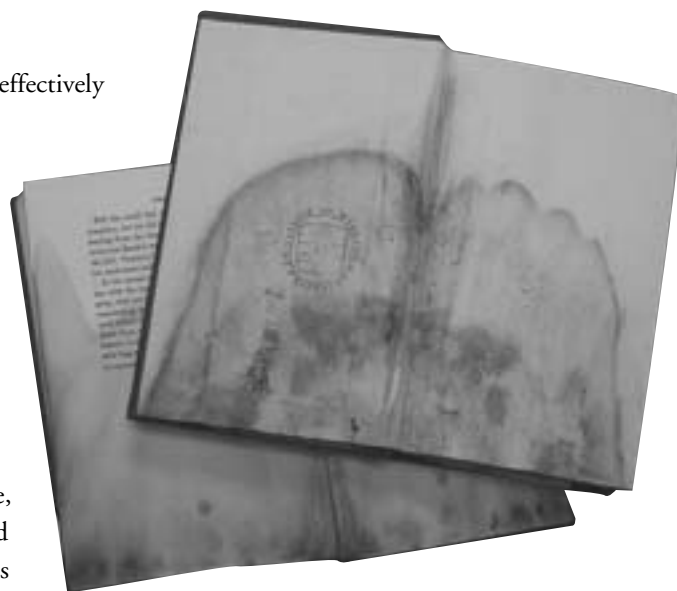
An example of the discoloration and “fuzzy bloom” of late-stage mildew contamination in a book.
